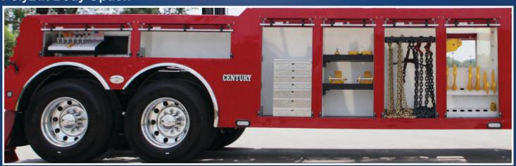
The PolyBilt body option provides a rugged durable design that has gone though years of field testing. The boxes feature roll up aluminum doors with remote lock/unlock, adjustable shelves and built in storage for your forks and popular attachments. The PolyBilt body is ideal for harsh environments to provide superior protection from rust and corrosion caused by road chemicals.
